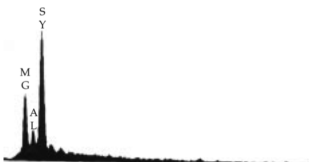
Figure 5. Elemental analysis of the inorganic particles
